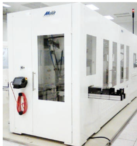
FIGURE 3. The Meikle Automation IS360 Wafer Inspector (top) uses NIR backlighting to detect and measure micro-cracks. The system incorporates DALSA Piranha and Eclipse linescan cameras, which interface to National Instruments Camera Link and LVDS frame grabbers that are installed in high-speed image-processing PCs. The PCs run Meikle's MASS material-handling and image-processing software. Standard encoder-based image acquisition along with continuous light and speed control ensures consistent image quality. Parallel processing is required to achieve one-wafer-per-second throughput (bottom).
